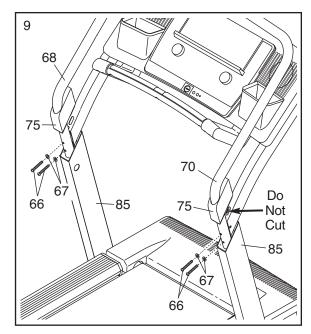
Press the right Upright Cover (75) onto the right Upright (85). Attach the Upright Cover with a 3/4" Screw (7).
